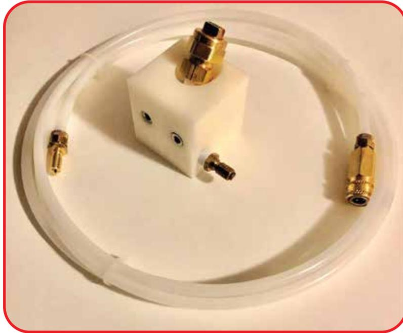
The **Delrin® Nozzle Cube Spray Assembly** promotes lubricant application to a precise location of the die by attaching the Delrin® Cube on or near the die. The spray line has a quick connect/disconnect fitting that plugs into the Delrin® Cube . The other end attaches to a lubrication system's pump for quick set up and tear down.
